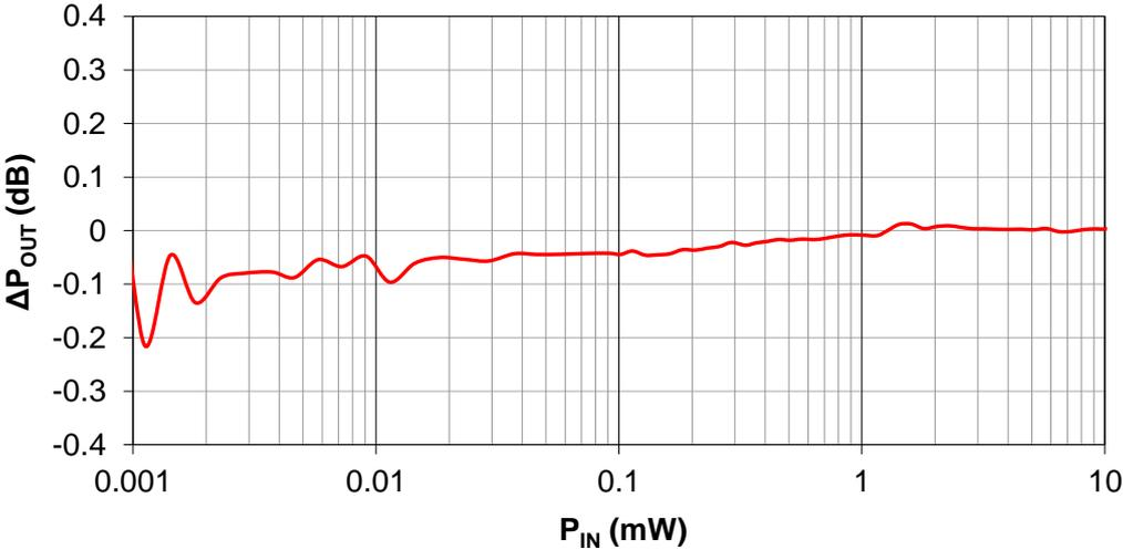
Fig. 6. Typical PS112 linearity error for digital outputs.
