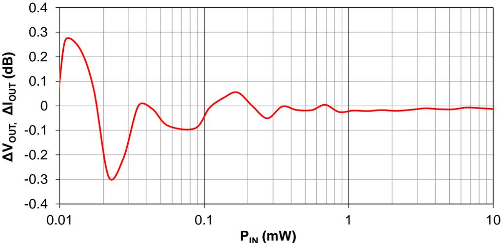
Fig. 5. Typical PS112 linearity error for analog outputs 0 – 10 V, 4 – 20 mA.
