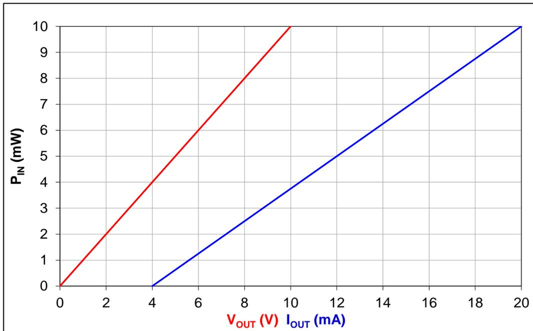
Fig. 3. Nominal PS112 transfer curves for analog outputs 0 – 10 V, 4 – 20 mA.
