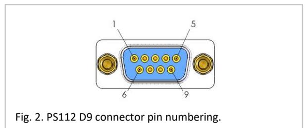
Fig. 2. PS112 D9 connector pin numbering.
