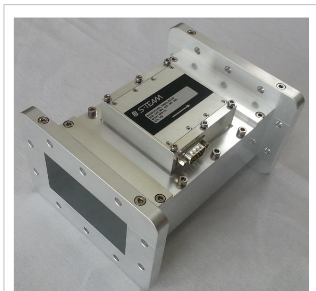
Fig. 2. BPM112 (version without LCD display) installed on a standard-length waveguide.
