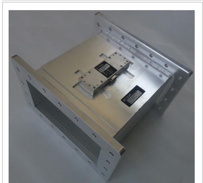
Fig. 2. BPM214 (version without LCD display) installed on a standard-length waveguide.
